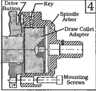
• Check to make certain face of the draw bar adapter is not bottomed against the inside face of the spindle Arbor (see figure 3 & 4).
